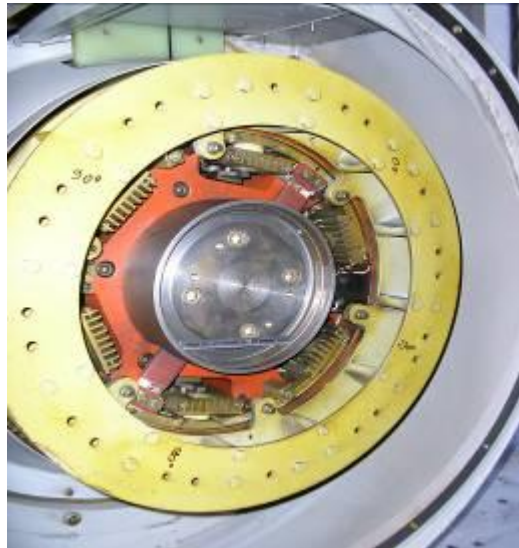
Figure 3 Shaft End Hole Pattern & Surrounding Diode Wheel
