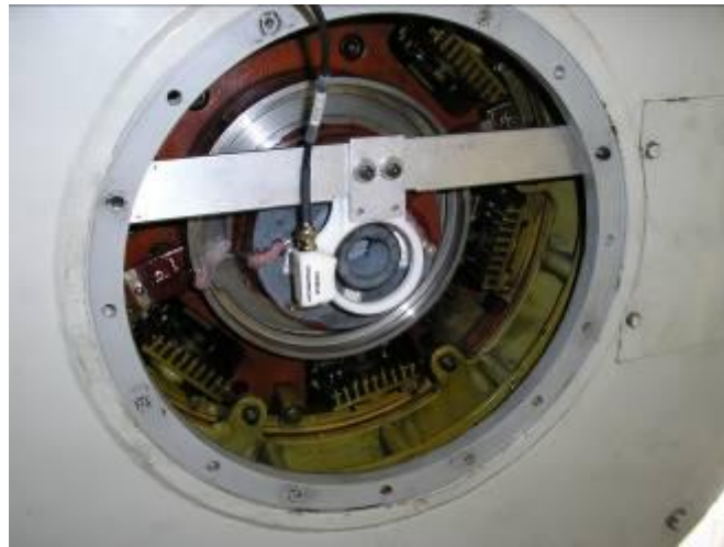
Figure 5 Mounted Adaptor Plate, Transmitter & Receiver Pickup Loop
