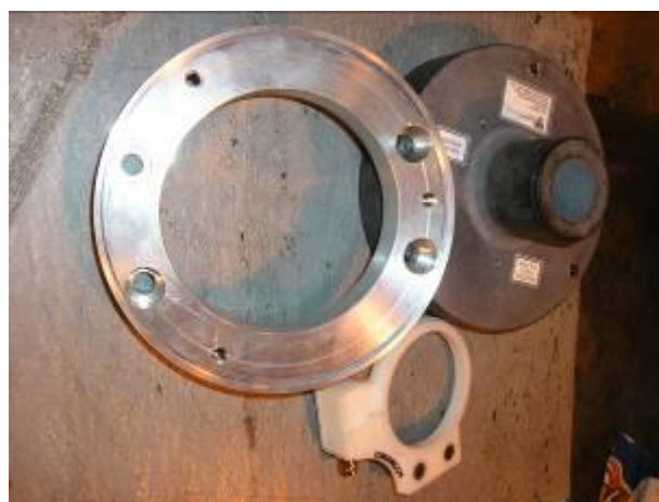
Figure 4 Adapter Plate, EFREM Transmitter “Top Hat” & Stationary Pickup
